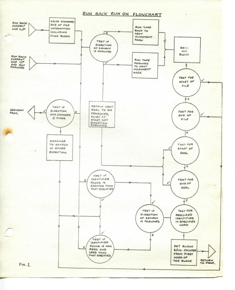
(d) If the search fails the direction of search is changed (up to six times) and the search continued. This is to avoid errors caused by the magnetic tape system misreading or failing to recognise alignment marks. The number of changes of direction allowed may be varied as experience dictates. If the programmer is uncertain of the direction in which a specified alignment mark lies, a 'Run-Back' instruction should be given, and the Master Program will change the direction of search if required.
